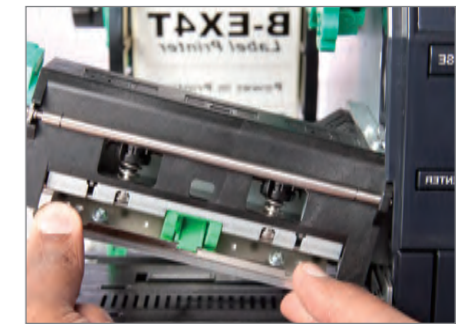
“卡扣式”打印头使装卸耗时降至最低
